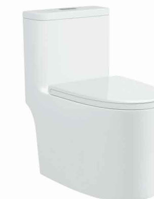
R248 Siphonic One Piece Toilet Size: 680 × 400 × 740mm S-trap, 300mm Roughing-in Vortex Flush
