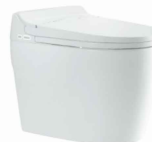
R2209B Foot Touch Flushing R2209C Automatic Cover All-in-one Toilet Size: 670 × 380 × 510mm S-trap:300,400 mm roughing-in P-trap:180 mm roughing-in Siphonic flushing
