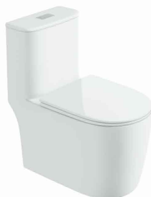
R149 Siphonic One Piece Toilet Size: 680 × 390 × 760mm S-trap, 300mm Roughing-in
