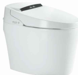
R2014B Foot Touch Flushing R2014C Automatic Cover All-in-one Toilet Size: 680 × 410 × 520mm S-trap:250,300 mm roughing-in P-trap:180 mm roughing-in Siphonic flushing
