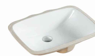
BT822 Under counter Basin Outside: 555 × 380 × 190mm Inside: 505 × 330mm
