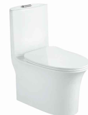
R239 Siphonic One Piece Toilet Size: 685 × 375 × 780mm S-trap, 300mm Roughing-in Vortex Flush
