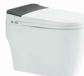
R2213B Foot Touch Flushing R2213C Automatic Cover All-in-one Toilet Size: 670 × 380 × 490mm S-trap:300,400 mm roughing-in P-trap:180 mm roughing-in Siphonic flushing
